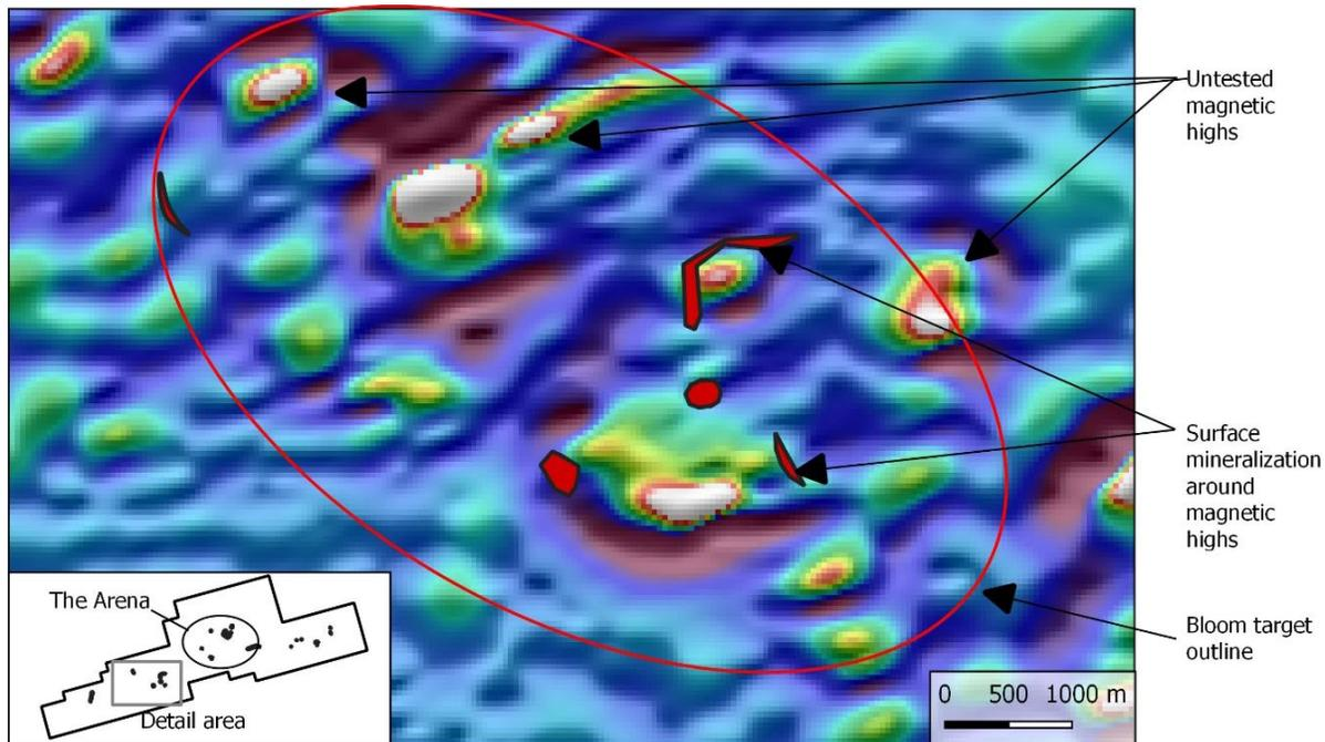
Figure 1. The Bloom Target overlain on a 1<sup>st</sup> vertical derivative magnetic map. Several magnetic highs are untested.
